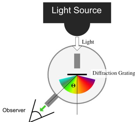
Figure 2: Setup of the Lab
